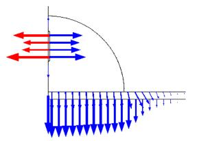
In the following graph the interface (red line) is seen after 0.1 s of applying 200 V (the drop is contracting).
