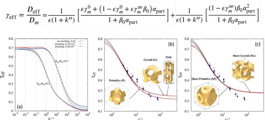
FIGURE 2. (a) Analysis of the random packings. Comparison between non-touching and touching spheres. (b)-(c) Analysis of monolithic silica columns: blue points represent experimental data[4], while red curves show the predictions of the approximate model. Curves for Gyroid G and TSM are not distinguishable.
