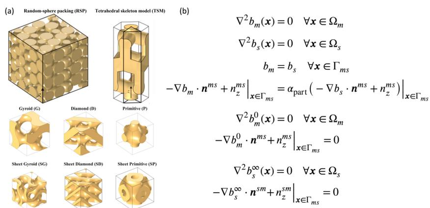
FIGURE 1. (a) Geometries adopted for modelling the unit-cell of the stationary phase: random packings of spheres (RSP), TSM, TPMS monoliths. (b) Stationary diffusion equations of the b-fields with related boundary conditions. Periodic boundary conditions must be also taken into consideration.
