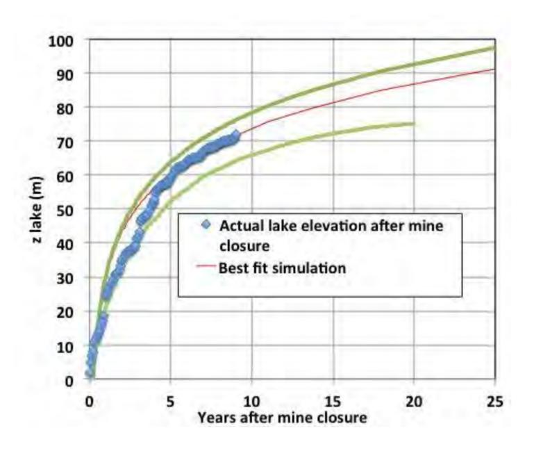
Sensitivity analysis (green lines) has shown permeability and storativity as most critical parameters for an accurate prediction.
