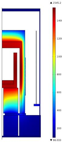
**Figure 2:** Fig.2: Temperature distribution in mock-up . Temperature distribution (Temperature in degree celsius) in mock-up equipment after two hours
