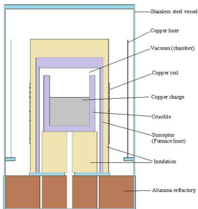
**Figure 1:** Fig.1: Schematic model of mock-up induction furnace
