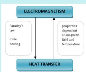
Fig. 2: Coupling of different fields in induction heating.
