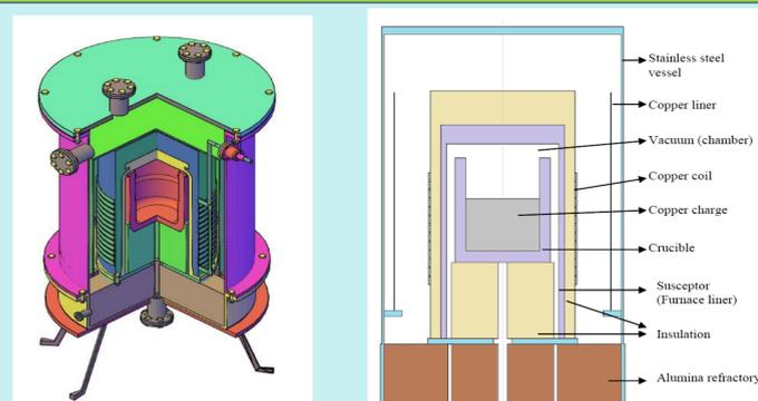
Fig.1: 3D and 2D schematic models of mock-up induction furnace
