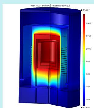
Fig. 7: 2D and 3D temperature distribution in mock-up induction furnace after 2 hours.
