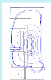
Fig. 6: Magnetic flux density inside the furnace.
