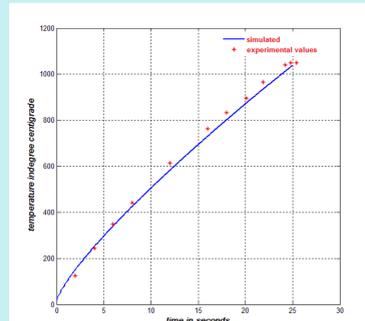
Fig.5: Experimental and simulated temperatures at 5mm from the top of work-piece in validation model.
