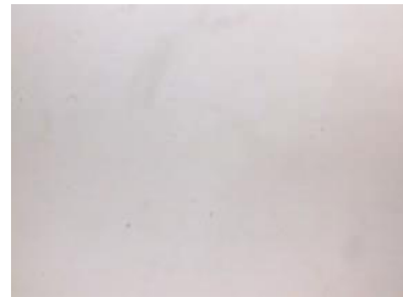
After ECMP : Ra 0.02 \mu\text{m}
