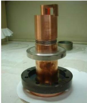
50 kW , 350 MHz peak peak power Coaxial loop coupler of 40 mm dia. and 150 mm length
