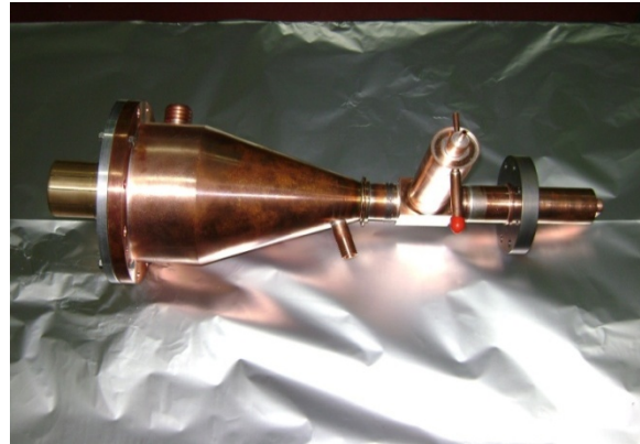
50 kW CW , 350 MHz Coaxial loop coupler of 155 mm dia. and 400 mm length
