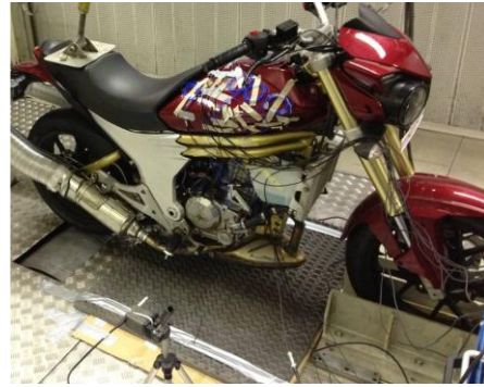
Figure 5. Noise measurement set-up
