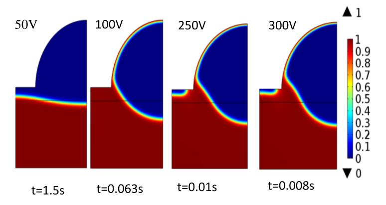
Simulations were done till 1.5s for a range of voltages while keeping the contact angle between the polymer and the upper electrode material at  $\theta_E$ = 10° to study the minimum time required for pattern transfer.
