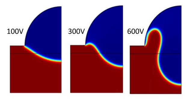
Nonwettable upper electrode surface was taken and simulations were done till 1.5s for a range of voltages while keeping the contact angle between the polymer and the upper electrode material at  $\theta_E = 170^{\circ}$ .
