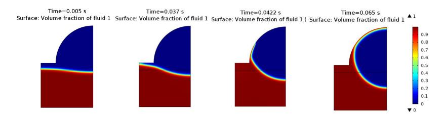
Voltage=200V, Contact angle between top electrode and polymer =  $20^{\circ}$  (Red represents polymer and blue represents air)
