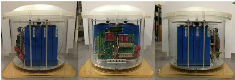
Figure 2: Physical Model of the Battery Power System
