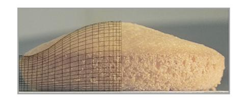
Final deformed meshing and real geometry
