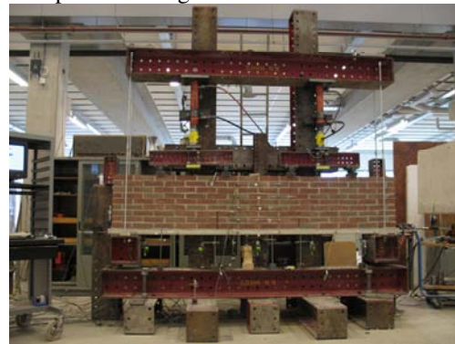
Figure 1. Lintel-wall test set-up
