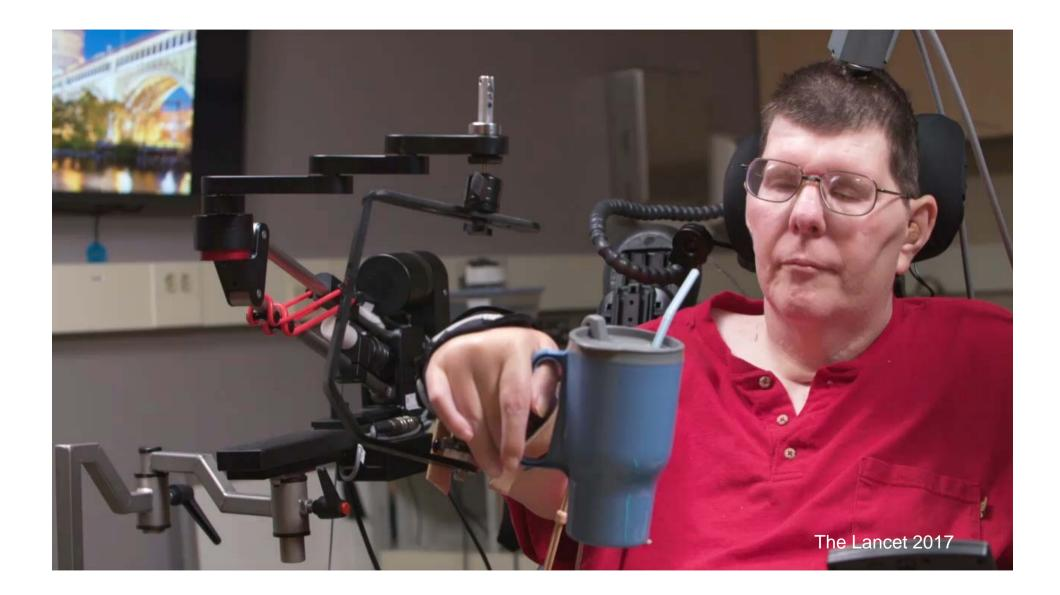
Sensor: 100 Microelectrodes Array 4 x4 mm
