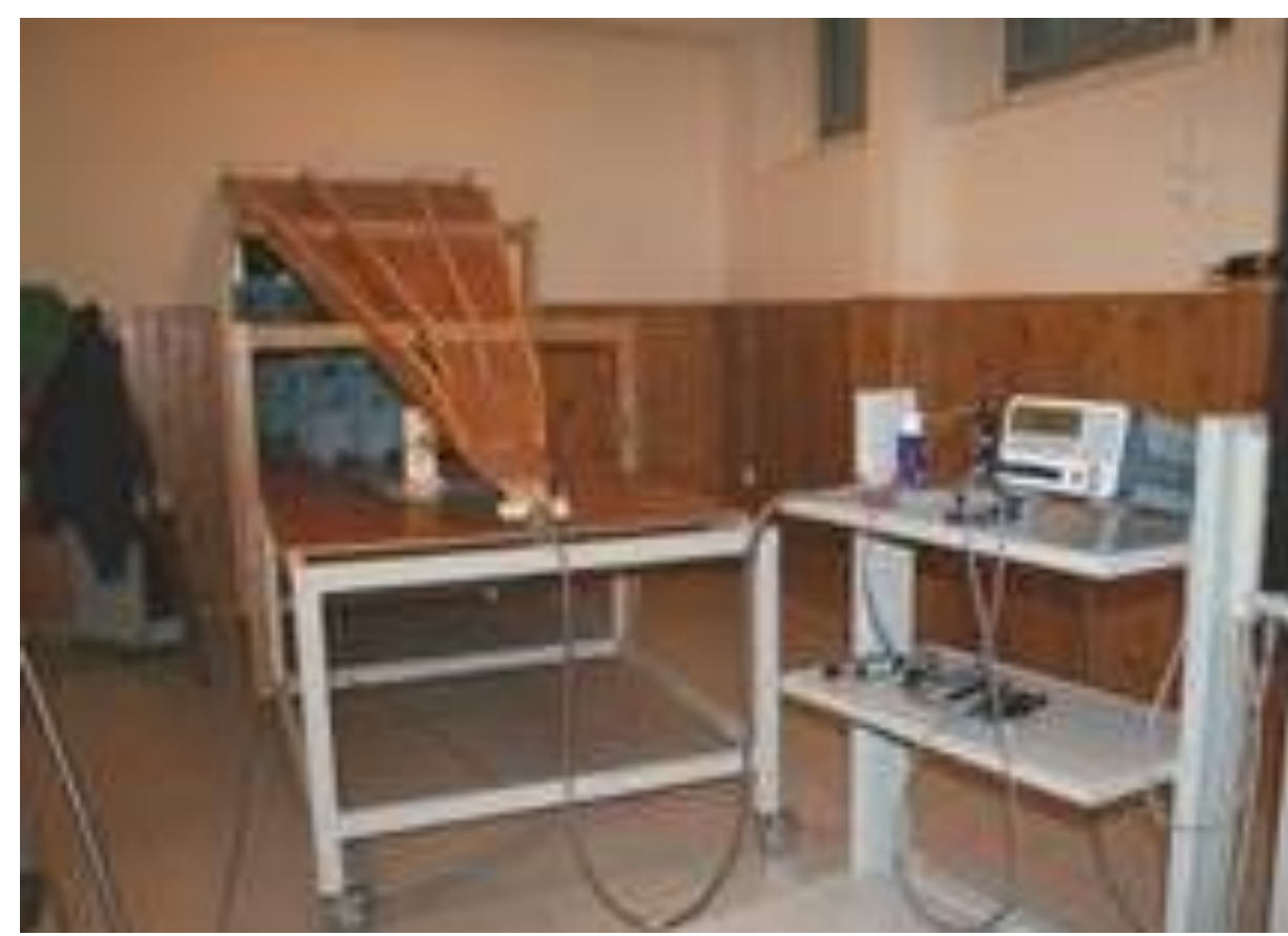
Figure 1. Open GTEM Cell
