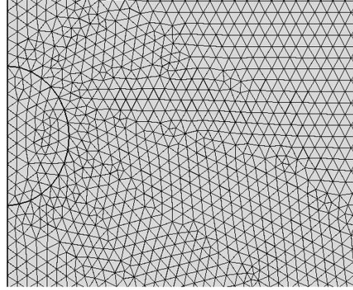
**Figure 2.** Mesh elements near the interface of the two phases
