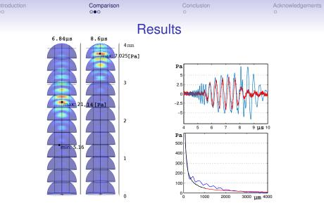
Left: output pressure field. Right top: comparison with experiment (red) at 4mm. Rgiht bottom: maximum pressure computed by multiple hemispheres (blue) versus computation by a hemisphere (black) with an extrapolation (red).
