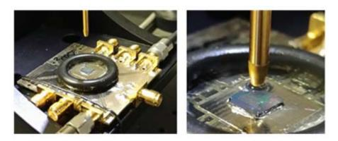
Output pressure measurements with a hydrophone (ONDA, HNC-1500) 3.8 mm away from the PMUT. The acoustic medium is Fluorinert FC-70 ( $\rho$  =1940 kg/m<sup>3</sup>, c =687 m/s).
