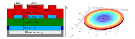
COSMOL model of a clamped multi-layer membrane resonator.
