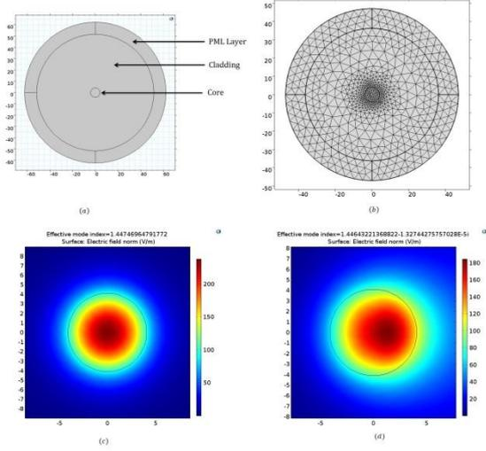
**Fig. 3:** (a) Cross-section of the optical fiber used in calculation of bend loss from COMSOL simulations. The core and cladding radius are  $3.05$  and  $62.5\mu\text{m}$  respectively. The PML thickness was taken to be  $7\lambda$ , (b) Physics controlled mesh with fine element size applied to the geometry, (c) LP01 mode propagating through the fiber when it is not bent, (d) LP01 mode when the fiber is bent at a diameter of  $10$  mm.
