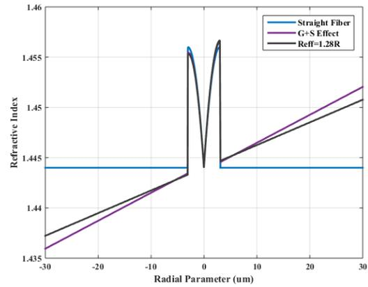
**Fig. 2:** Refractive index profile of the fiber, modelled with a central dip, for straight fiber and fiber bent at 10 mm diameter using GEBT and elasto-optic correction factor.
