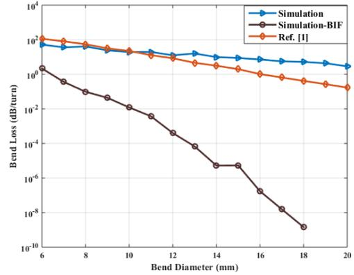
**Fig. 4:** Results of loss due to in-plane bending of the fiber in COMSOL simulations for both normal and bend insensitive fiber for bend diameters ranging from  $6 - 20$  mm. Also shown are loss calculated using formula given in reference [1].
