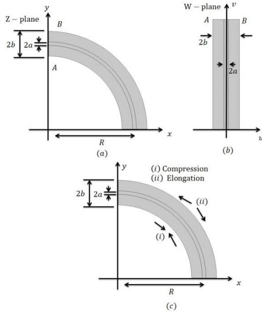
**Fig. 1:** (a) Schematic of the bent fiber, (b) Mapping of curved waveguide to equivalent straight guide by conformal mapping, (c) Stresses experienced by fiber under bending condition
