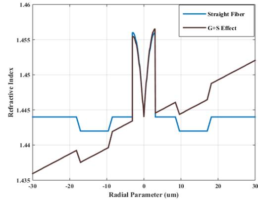
**Fig. 6:** Refractive Index of bend insensitive fiber (BIF) with a trench in cladding, (a) in unbent case and (b) fiber bent at 10 mm bend diameter.
