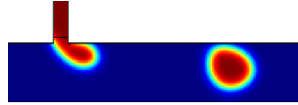
Figure 3: Droplet formation at \sigma = 15 mN/m at t=4 ms.
