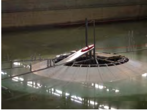
Figure 1. Picture of the experimental model of the conical island with the landslide body.
