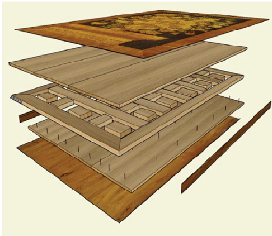
Figure 1. Exploded view of the construction of one cabinet door (Source: Rijksmuseum, Amsterdam)
