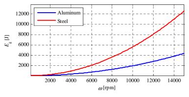
Figure 3. Energy stored with respect to the rotational speed for the considered flywheels
