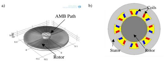
Figure 5. Generated geometries: a) complete flywheel rotor; b) AMB
