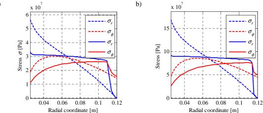
Figure 2. Radial (blue) and azimuthal (red) stress components for initial (dashed line) and optimized (solid line) flywheel profiles calculated at 1500 rpm. a) aluminum; b) steel
