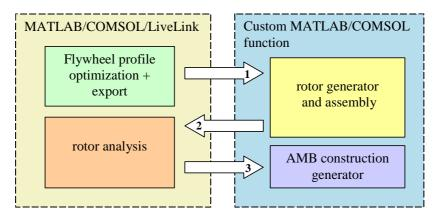
Figure 4. Path for automatic generation of flywheel components.
