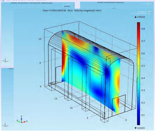
The internal air temperature gradients are important and produce a complex air flow distribution due to the mix between the natural convection, connected to buoyancy forces and the air density variation, and the forced convection provided by the operating fan-coils unit.
