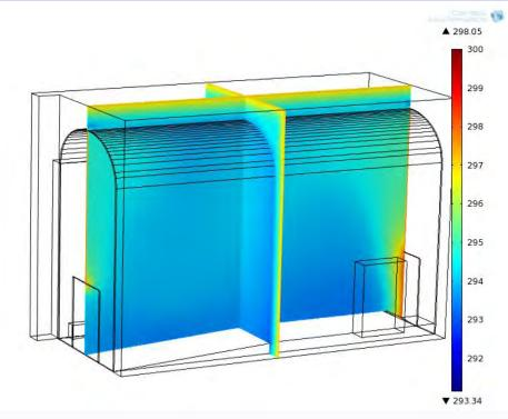
Taking into account that during the door opening and closing, the passage of a person needs about five seconds, the external air flow rate is 1.4 m³/s during the hottest hours and 0.19 m³/s in the remaining hours of the day. In particular, at the h 14 (the hottest hour) when the door is open, the three fan-coils unit needs a cooling peak power of 25.5 kW. For the door closed condition, during the whole day, the cooling peak power requested by the plant is 13.7 kW.
