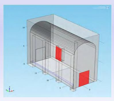
This thermal buffer, actually called *hot room*, was considered as one-zone model made by the large glazed surfaces supported by steel profiles connected to the structure.
