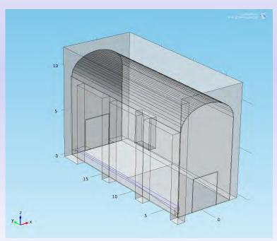
This thermal buffer, actually called *hot room*, was considered as one-zone model made by the large glazed surfaces supported by steel profiles connected to the structure.
