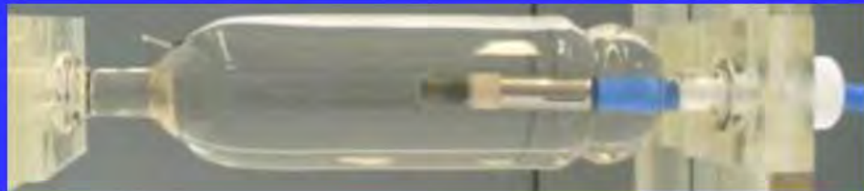
Vessel with an ion chamber
