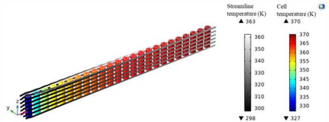
Figure 8. Temperature distribution results at 7.5C discharge rate
