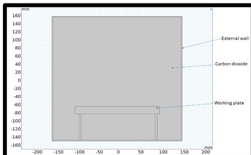
Figure 2. 2D geometry of the SpaceQ model (in mm)
