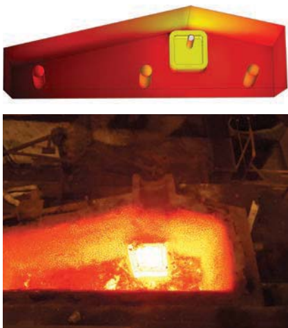
FIGURE 3. Model of a tundish using the CFD Module in COMSOL Multiphysics (top) and actual tundish during emptying of molten steel (bottom).
