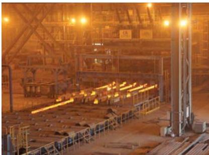
FIGURE 1. Discharge table of the continuous caster showing solidified strands being cut and discharged.
