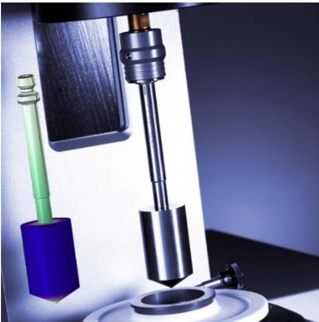
Figure 1 : A typical concentric cylinder measuring setup and its COMSOL® simulated eigenfrequency mode.
