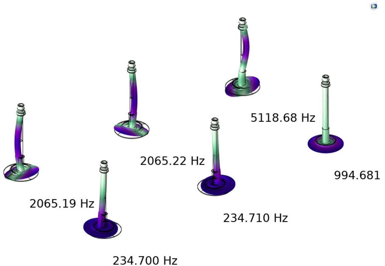
Figure 4 : COMSOL® array visualization of mode shapes for different eigenfrequencies for a Cone-Plate CP50-1 – not all are torsional relevant.
