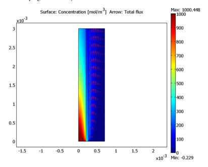
Figure 6: Concentration and flux in the three subdomains.
