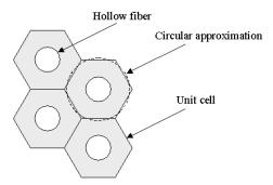
Figure 3: Hexagonal-shaped unit cell of the fiber assembly.
