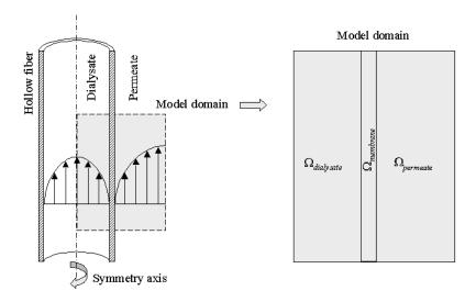
Figure 2: Diagram of the dialysis fiber.
