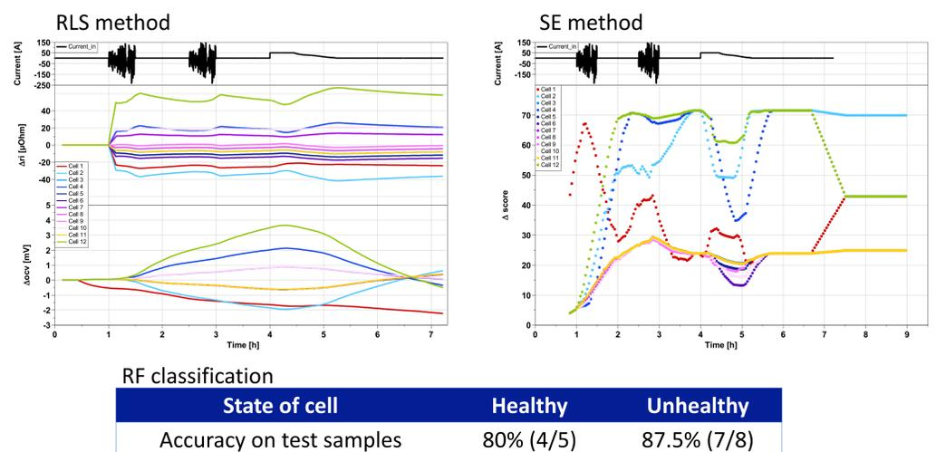
FIGURE: Overview of the studied algorithms for the fault diagnosis method with the respective results
