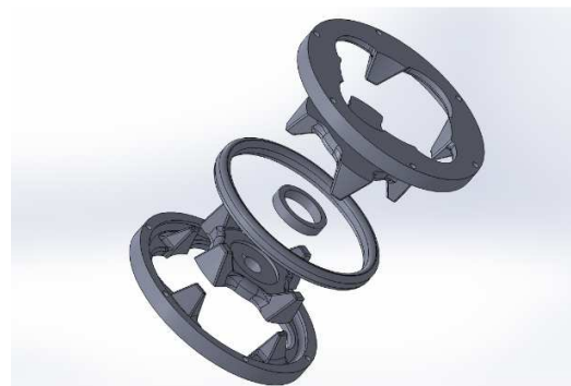
Figure 1: Exploded view of 1 phase claw pole.
