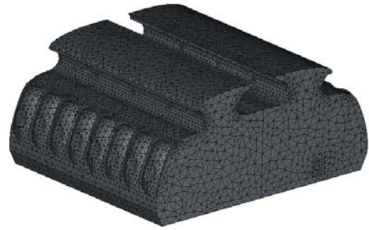
Fig. 5: FE model of the cavity
