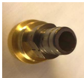
Figure 2: A photograph of the DFEA cathode brazed on an HBESL cathode. The emitter area is the dark circular area on the plug surface.
